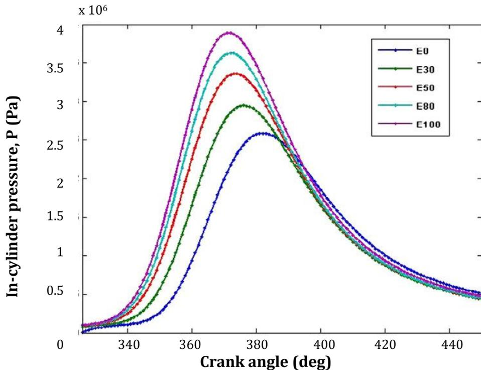
**Figure 3.** In-cylinder pressure against the crank angle for different ethanol-gasoline blends [6]
