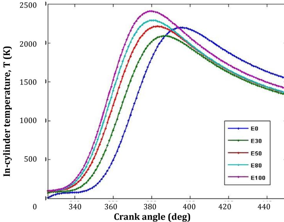
**Figure 4.** In-cylinder temperature against the crank angle for different ethanol-gasoline blends [6]
