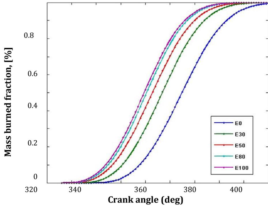
**Figure 5.** Mass burned fraction vs. crank angle for different ethanol-gasoline blends [6]
