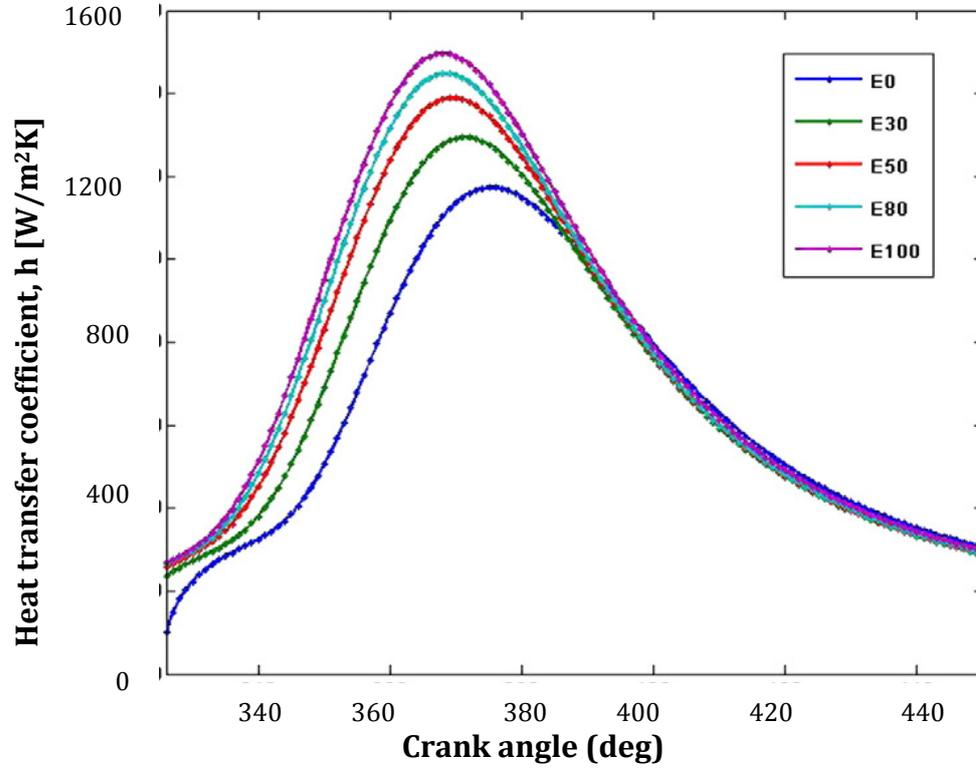
**Figure 6.** Coefficient of heat transfer vs. crank angle for different ethanol-gasoline blends [6]
