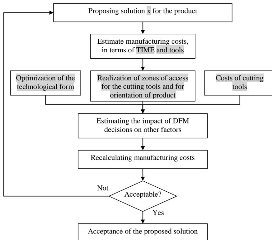
**Figure 7.** Example of applying of the DFM algorithm
