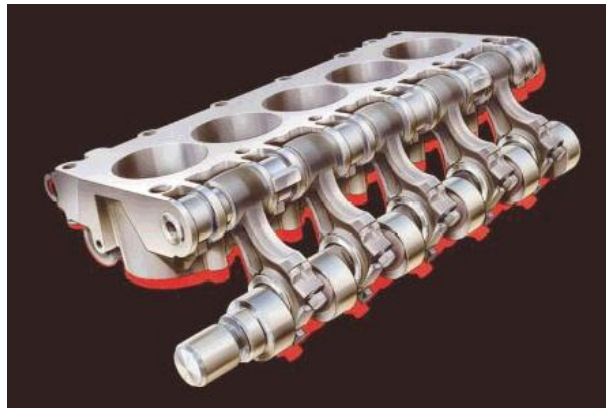
Figure 3. Eccentric shaft mechanism controls the CR [6]
