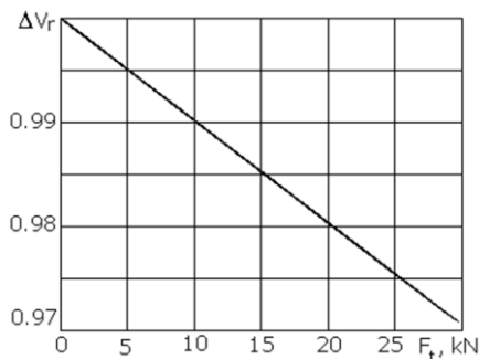
Figure 6. Variation of the coefficient of speed reduction \Delta V_r considering the drawbar pull F_t .
