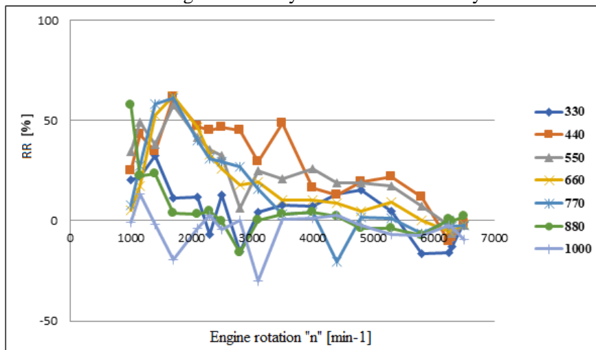
Figure 7. Relative reductions in NOx concentrations between optimized VVT and zero VVT
